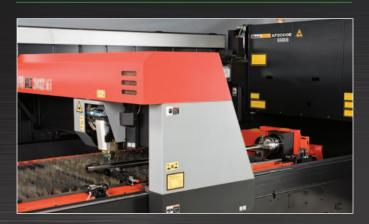
Providing for quick and efficient processing of round and square tubing, an optional rotary axis further enhances the capabilities of the FOM2.
